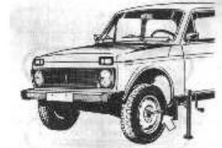
Fig 53. Jacking up car for replacement of wheels.
