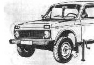
Fig 53. Jacking up car for replacement of wheels.
